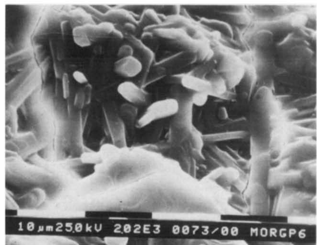
Fig. 6. Silicon nitride oxidized at 1200°C. Partial pressure of water vapour in the air flow equal to 50 kPa.
